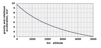
Fig. 6. Gravity minus centrifugal acceleration versus altitude
