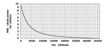
Fig. 2. Power needed for a 5 ton climber climbing at 200 m/s
