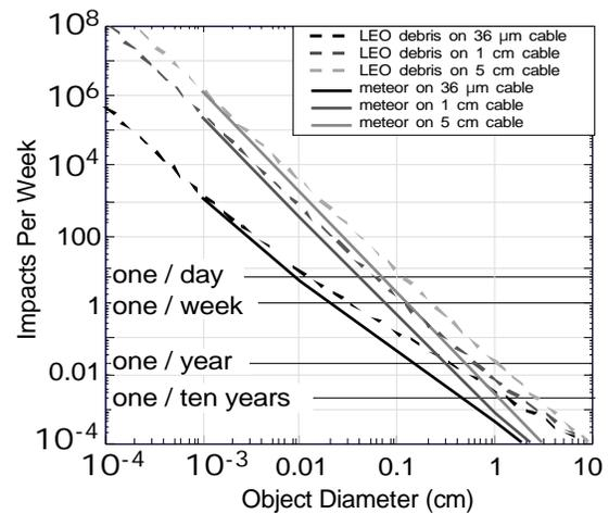
FIG. 5: Impacts per week average for various particle and cable dimensions. Based on meteor flux data <sup>21</sup> and LEO debris data <sup>22</sup>.
