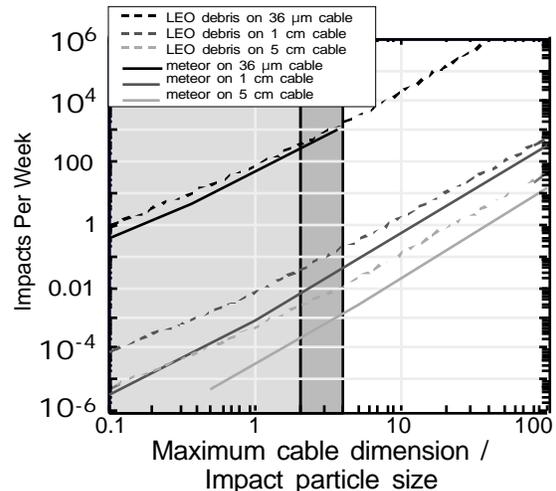
FIG. 6: Plot of Impacts per week versus the ratio of maximum cable dimension to the size of the impacting object. If the object is one half the maximum cable dimension the cable will be severed. Objects with diameters up to and beyond one quarter the maximum dimension of the cable may sever it. Based on meteor flux data <sup>21</sup> and LEO debris data <sup>22</sup>.
