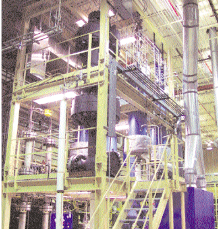
Figure 6. This pilot plant produces single-wall carbon nanotubes by a high-pressure carbon monoxide flow method and is expected to produce thousands of kilograms a week by 2005.
